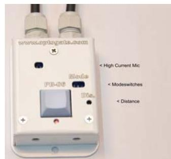
\*\*If you are using very high current mics, set the two dip switches in upper left face plate to the off-down position otherwise leave them "up"
